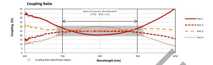
Coupling ratio (%) is the ratio of the optical power from each output port to the sum of the total power of all output ports as a function of wavelength.
