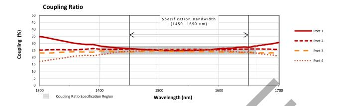
Coupling ratio (%) is the ratio of the optical power from each output port to the sum of the total power of all output ports as a function of wavelength.
