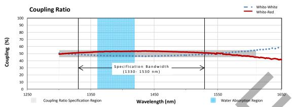
Coupling ratio (%) is the ratio of the optical power from each output port to the sum of the total power of both output ports as a function of wavelength. It is not impacted by the water absorption region because both output legs are affected equally.
