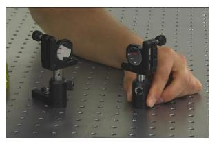
**Figure 1**. The beam path reflected by these two mirrors depends on their orientations with respect to one another.
