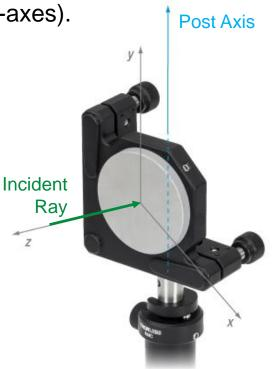
**Figure 13**. The *x*-, *y*-, and *z*-axes of the global coordinate system.
