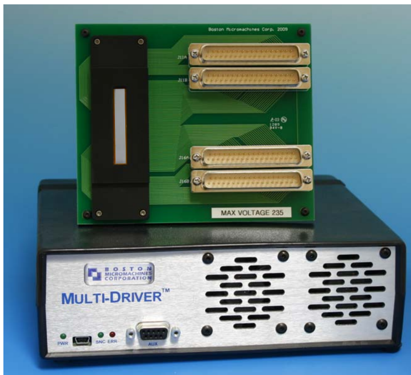
Figure 13. Linear Array DM Prototype system with 14-bit Multi-Driver electronics.
