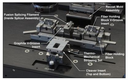
Each labeled component above can be purchased separately to configure the workstation for various fiber types.
