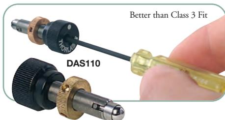
The DAS110 is a standard 1/4"-80, 1.00" long adjuster screw with an internal differential adjustment mechanism. The fine adjustment is actuated by inserting a hex wrench through the clearance hole in the adjuster knob. Every rotation of the DAS110 fine adjustment mechanism yields a highly demagnified displacement of just 25 µm/rev. This adjuster is ideal as a drop-in replacement for increasing the resolution on most Thorlabs' mirror mounts.
