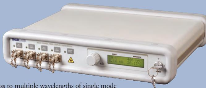
Thorlabs' 4-Channel, Fiber-Coupled Laser Source provides easy access to multiple wavelengths of single mode (SM) fiber-coupled light. The laser source is configured to accept any combination of four SM fiber-pigtailed laser diodes; choose from the following wavelengths: 406, 473, 488, 635, 658, 670, 785, 808, 850, 904, 980, 1310, 1550 nm. More wavelengths will be made available in the future. Please check our website for the latest details.
