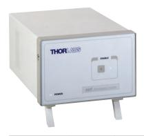
The BSC101 apt<sup>TM</sup> controller is a single-channel 50 W stepper motor controller designed to drive high-power, 2-phase bi-polar stepper motors, with or without encoder feedback. It has been designed to drive the higher power stepper motor equipped nanopositioning actuators and stages offered by Thorlabs as well as any generic two-phase bi-polar motor of varying powers and varying cardinal step sizes, making this a very flexible unit.
