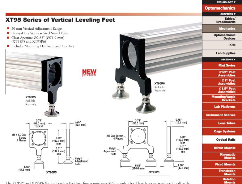
The XT95P5 and XT95P6 Vertical Leveling Feet have four countersunk M6 through holes. These holes are positioned to allow the leveling feet to be attached to the ends of XT95 rails using the included 5 mm hex key and four M6 x 1.0 cap screws. In order to allow access to the interior of the optical rail, each leveling foot has a hole with a Ø2.83" (Ø71.9 mm) clear aperture.
