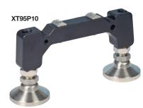
All of the leveling feet can be adjusted over a vertical range of 30 mm (1.18"). Once the correct height is set, a locking nut can be tightened to prevent further adjustment. The durable stainless steel swivel pads ensure that the leveling feet maintain stable contact with the surface they are resting on, even if the surface is tilted.
