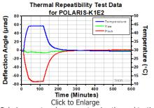
Each Polaris mount undergoes extensive thermal testing to ensure high-quality performance. Please see the *Test Data* tab please refer to the *Design Features* tab for detailed information. for additional test results.
