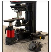
MCM3001 Being Used to Control Both Axes of the PLS-XY and one ZFM2020 Focusing Module
