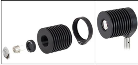
From left to right are shown an uncoated plano-convex calcium fluoride lens, an HEP3965 bulb, the HEPM mounting adapter, an HSLT2 heat sink lens tube, and an LMR2(/M) fixed optic mount. Electrically insulating thermal compound (not shown) must be used between the bulb and mounting adapter for proper heat dissipation.
