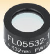
FL05532-1 Ø1/2" Filter CWL = 532 nm, FWHM = 1 nm
