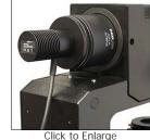
The MWWHL4 LED and COP1-A microscope collimation adapter used as a trans-illumination source for an Olympus microscope.
