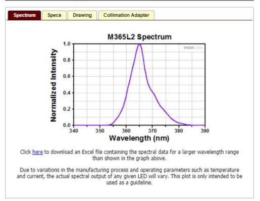
M365L2 - 365 nm, 190 mW (Min) Mounted LED, 700 mA
