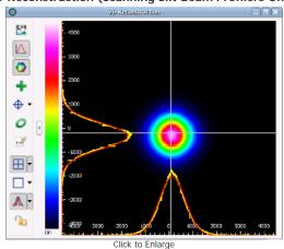
Slit beam profilers only measure two real orthogonal cross sections of the beam (i.e., the
