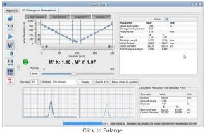
The beam diameter and location of the beam waist are shown after an M² analysis has been performed. Note: This functionality is only enabled when one of the M² analysis systems is connected to the PC.
