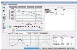
Click to Enlarge The divergence of the beam is shown after an  $M^2$  analysis has been performed. Note: This functionality is only enabled when one of the  $M^2$  analysis systems is connected to the PC.
