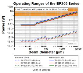
These maximum and minimum beam power limits are provided as functions of  $1/e^2$  beam diameter for knife-edge and scanning-slit measurements and may not apply to measurements of total power. Please see the scanning-slit beam profiler page for more information. To prevent thermal damage to the measurement head, do not operate for longer than 5 s with input powers exceeding 1 W.
