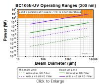
Click to Enlarge The neutral density filter will begin to heat up and can be damaged if exposed to incident powers above 1 W for more than a few seconds.
