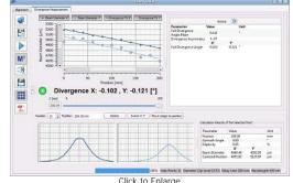
Click to Enlarge The divergence of the beam is shown after an M<sup>2</sup> analysis has been performed. Note: This functionality is only enabled when one of the M<sup>2</sup> analysis systems is connected to the PC.
