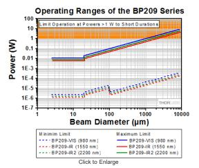
These maximum and minimum beam power limits are provided as functions of 1/e<sup>2</sup> beam diameter for knife-edge and scanning-slit measurements and may not apply to measurements of total power. Please see the scanning-slit beam profiler page for more information. To prevent thermal damage to the measurement head, do not operate for longer than 5 s with input powers exceeding 1 W.
