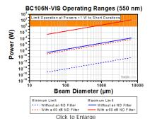
Click to Enlarge The neutral density filter will begin to heat up and can be damaged if exposed to incident powers above 1 W for more than a few seconds.
