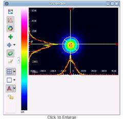
Click to Enlarge The 2D Projection graph shows the image from the Beam Profiler indicating the power intensity distribution within the selected Region of Interest (ROI). Buttons along the side allow users to save the image, show or hide the x and y scales, mark the centroid or peak positions, and display an approximated Beam Ellipse superimposed on the image.
