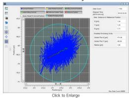
The Beam Stability Window allows the stability versus time to be recorded and viewed. Display options include the Centroid Positions, Latest Plotted Centroid, Rolling Centroid Positions, Reference Positions, and Smallest Enclosing Circle.
