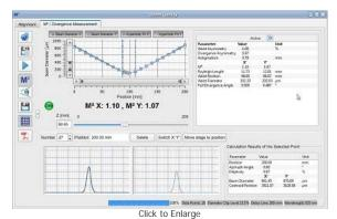
The beam diameter and location of the beam waist are shown after an M<sup>2</sup> analysis has been performed. Note: This functionality is only enabled when one of the M<sup>2</sup> analysis systems is connected to the PC.
