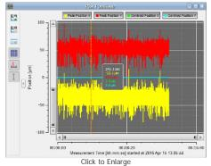
The positions of the X and Y peak and X and Y centroid positions can be displayed as a function of time in this window.
