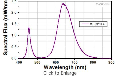
Broadband LED Spectra Scaled to Min Power
