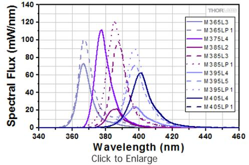
Visible LED Spectra Scaled to Min Power
