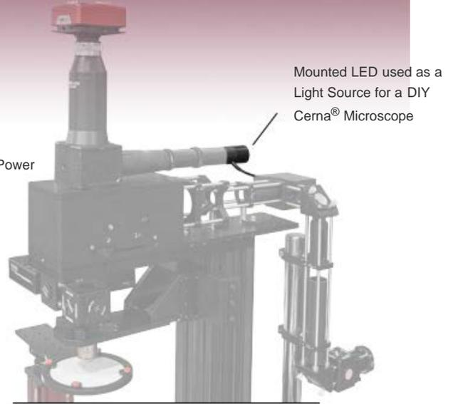
Mounted LED used as a Light Source for a DIY Cerna® Microscope
