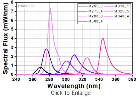
UV LED Spectra Scaled to Min Power
