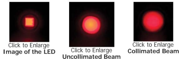
3. Once the proper collimation position of the lens has been found, lock the position of the lens in place.
