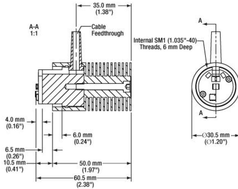
This LED features a Ø30.5 mm heat sink.
