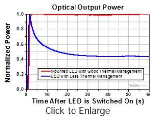
by the LED after it is turned on is typical behavior during the first few minutes of operation. It corresponds to the period of time required for the LED to warm up to the point where it is thermally stable. Please note that this graph represents the performance of a single LED; the performance of individual LEDs will vary within the stated specifications.
