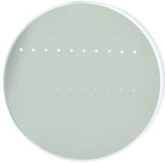
The photograph above is a protected aluminum-coated mirror after LIDT testing. In this particular test, it handled  $0.43 \text{ J/cm}^2$  (1064 nm, 10 ns pulse, 10 Hz,  $\text{Ø}1.000 \text{ mm}$ ) before damage.
