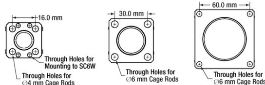
An example of the standard cage plate measurements determining cage system compatibility.
