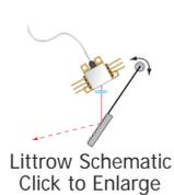
Lasers consist of an active gain element and optical feedback to this gain element. The most common diode lasers are based on a Fabry-Perot design with a linear waveguide and reflective surfaces at both ends of the gain chip to provide feedback. Some Fabry-Perot lasers
