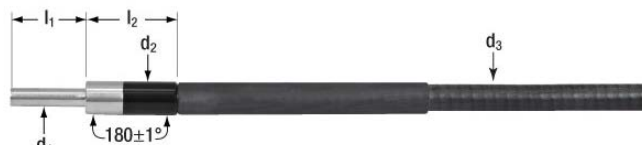
Figure 7: End portion of an LLG with Key Dimensions Labeled.
