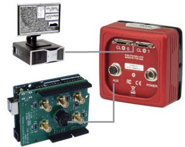
Click for Details A schematic showing a TSI-IOBOB2 connected to an Arduino in a custom camera system.
