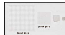
Click to Enlarge Close Up of the Four Grid Patterns on the R1L3S3P Target
