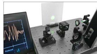
Click to Enlarge Loud music with a strong bass line causes fluctuations in the interference pattern.
