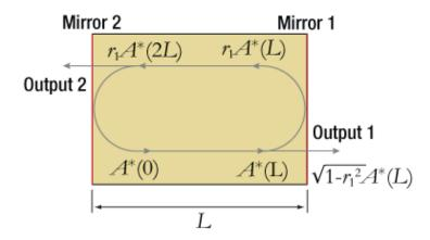
Figure 1: Fabry-Perot Laser Structure
