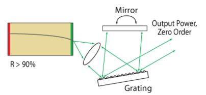
Figure 6: Littman-Metcalf External Cavity Laser
