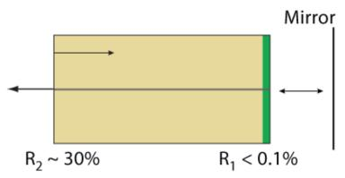
Figure 3: External Cavity Operation Based on a Gain Chip
