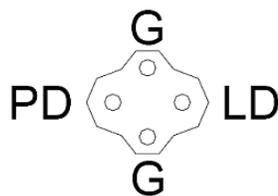
Figure 2. TCLDM9 Standard Configurations
