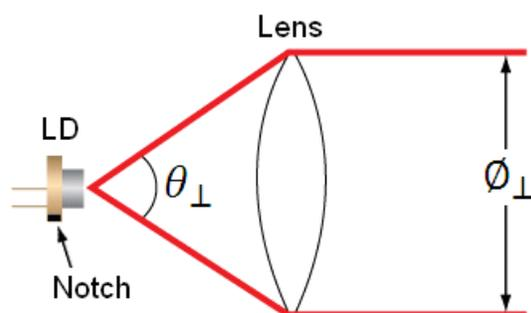
Figure 1. Perpendicular beam divergence from L785P025 style A laser diode
