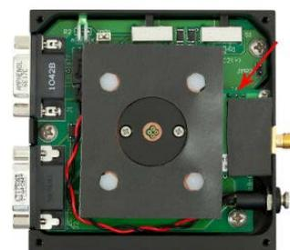
Figure 3. TCLDM9 Internal Circuitry Showing Jumper J4
