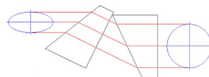
**Figure 3.** Anamorphic Prism Pair and optic trace for an ellipse to round beam.
