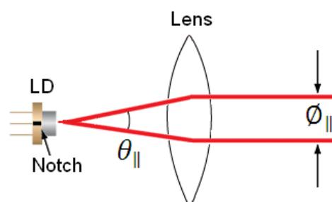
Figure 2. Parallel beam divergence from L785P025 style A laser diode
