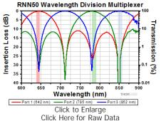
This plot shows an example of the spectral performance of a RNN50 3-wavelength WDM. The lines represent the spectral response of each channel, while the colored regions denote the bandwidth around the center wavelengths. This data is typical; performance of each WDM may vary from unit to tunit. Data was obtained without connectors.
