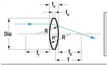
Focal Length f: fh: **Back Focal Length** Front Focal Length ff: **Radius of Curvature** R: **Center Thickness** tc: **Edge Thickness Back Principal Plane** H": Dia: Diameter
