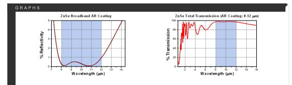
Shown above is a graph of the theoretical percent reflectivity of the AR coating as a function of wavelength. The average reflectivity in the 8 - 12 µm range is <1.5%. The blue shading indicates the region for which the AR coating is optimized.
