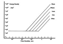
LIDT in energy density vs. pulse length and spot size. For short pulses, energy density becomes a constant with spot size. This graph was obtained from [1].
