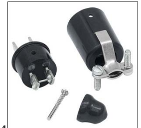
Step 4 Click to Enlarge Third, remove the protective cap to expose the short wire, which can be unsoldered.
