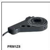
The central aperture of the PRM1Z8 rotation mount has a standard SM1 internal thread, for compatibility with a range of optics. Two SM1RR retaining rings are included to secure optical components in this aperture. The rotating platform features four 4-40 holes, four 8-32 (M4) holes and four 6-32 (M3) holes to allow for the addition of accessories. Please see the *Mounting* tab for all of the possible mounting options.
