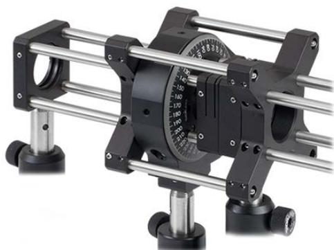
The PRM1Z8 can be aligned within a 30 mm cage system by using two LCP02 30 mm to 60 mm cage plate adapters, a CPR1 rotating cage segment plate, and three ER3 Cage Rods. This creates a motorized rotation mount within a rigid optical assembly. For more details on how the PRM1Z8 and CPR1 work together, please see the animation to the right.
