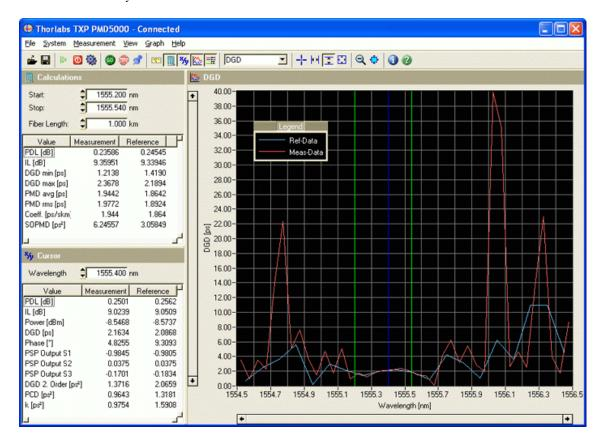
The green vertical lines show the wavelength range for which the analyzed parameters are calculated (upper left "Calculations" pane). The blue vertical line shows a specific single wavelength (cursor) for which the parameters are calculated (lower left "Cursor" pane).
