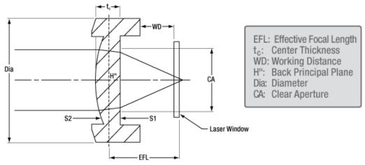
Please note the effective focal length is determined from the back principal plane, which does not coincide with the flat surface of the lens.
