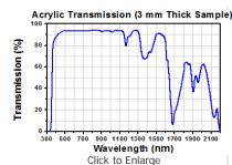
The transmission curve above shows total transmission through uncoated acrylic, including surface reflections. Our CAY046-A plastic aspheric lens is fabricated from this material and then an antireflection coating for 400 to 700 nm is deposited on the surface.
