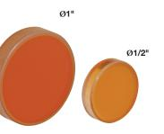
Thorlabs' Ø1/2" and Ø1" Zinc Selenide (ZnSe) PrecisionWindows are available either uncoated or with an AR coating for the  $8 - 12 \,\mu m$  range on both sides. Due to its wide transmission band and low absorption in the red portion of the visible spectrum, ZnSe in an ideal material for use in optical systems that combine CO2 lasers, operating at 10.6 microns, with HeNe alignment lasers.
