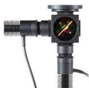
Figure 6.8 Two-LED source. This is the same as Example 1, but with the blue LED removed.
