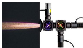
Figure 6.7 Beam Profile of Source with 3 Mounted LEDs
