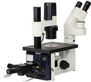
Click to Enlarge Figure 6.1 Multi-LED Source Coupled to Microscope Illumination Port
