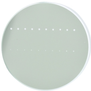
Figure 37A This photograph shows a protected aluminum-coated mirror after LIDT testing. In this particular test, it handled 0.43 J/cm 2 (1064 nm, 10 ns pulse, 10 Hz, Ø1.000 mm) before damage. According to the test, the damage threshold of the mirror was 2.00 J/cm 2 (532 nm, 10 ns pulse, 10 Hz, Ø0.803 mm). Please keep in mind that these tests are performed on clean optics, as dirt and contamination can significantly lower the damage threshold of a component. While the test results are only representative of one coating run, Thorlabs specifies damage threshold values that account for coating variances.
