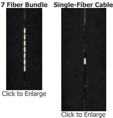
Left: Light exiting the end face of a BFL105HS02 linear bundle placed behind the 20 µm x 2 mm entrance slit of the CCS100 spectrometer. Right: Light exiting the end face of an M15L01 fiber patch cable placed behind the 20 µm x 2 mm entrance slit of the CCS100 spectrometer.
