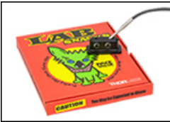
Click to Enlarge Diffuse Measurement Taken at 45° Using RPH Holder Block
