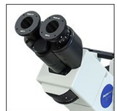
Two SM2Y2 adapters replace the lens elements of the trinocular eyepieces.
