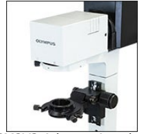
SM2Y3 Adapter Attached to Condenser Holder of Olympus IX71
