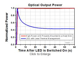
output power after the lifetime has elapsed. Thorlabs defines the lifetime of our LEDs as  $B_{50}/L_{50}$ , meaning that 50% of the LEDs with a given Item # will fall below 50% of the initial optical power at the end of the specified lifetime. For example, if a batch of 100 LEDs is rated for 150 mW of output power, 50 of these LEDs can be expected to produce an output power of ≤75 mW after the specified LED lifetime has elapsed.
