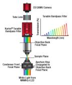
Click to Enlarge Schematic of the Hyperspectral Imaging Microscope
