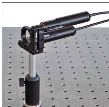
Click to Enlarge A KM100 mirror mount with the screw adjusters replaced by two ZST206 actuators.
