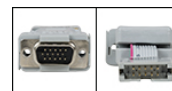
Click to Enlarge Connectors terminating the converter cable. The image on the left shows the high-density D-Type male 15-pin connector, and the image on the right shows the 10-pin male IDC socket connector.
