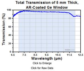
This graph shows the full scale measured transmission of an AR-coated germanium window at normal incidence. The shaded region denotes the AR coating range, over which  $R_{avg} < 1\%$  per surface.
