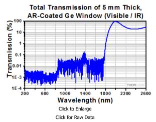
This graph shows the measured transmission of an AR-coated germanium window at normal incidence in the visible wavelength range. Please note that out-of-band transmission is not monitored during production and will vary from lot to lot.
