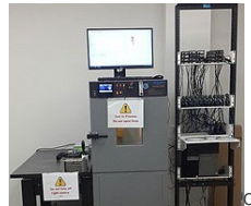
Click To Enlarge Damp Heat Testing Setup
