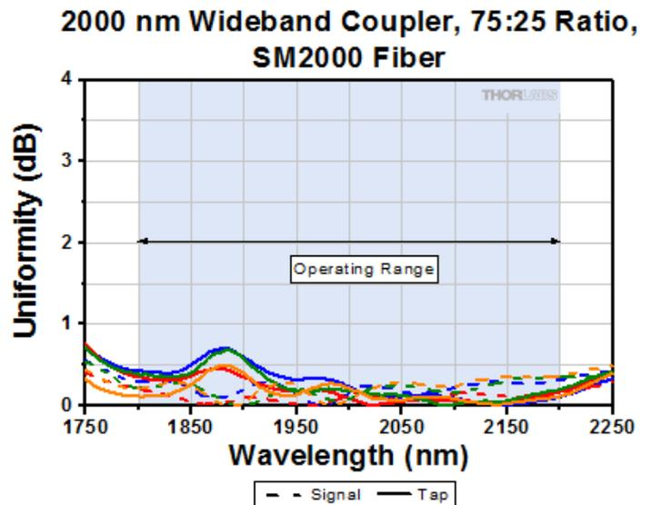
The plot above shows the uniformity measured at each output leg of four TW2000R3A2A couplers (tap and signal outputs from the same coupler indicated by matching colors). The blue-shaded region denotes the coupler's full operating wavelength range.
