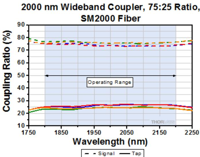
The plot above shows the coupling ratio measured at each output leg of four TW2000R3A2A couplers (tap and signal outputs from the same coupler indicated by matching colors). The blue-shaded region denotes the coupler's full operating wavelength range.
