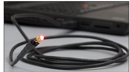
A LED630L being powered by the USB port in a laptop.
