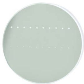
The photograph above is a protected aluminum-coated mirror after LIDT testing. In this particular test, it handled 0.43 J/cm 2 (1064 nm, 10 ns pulse, 10 Hz, Ø1.000 mm) before damage.
