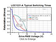
In addition, the material's viscosity and hence the switching speed also depend on temperature of the LC material. As can be seen below, the switching speed can increase by as much as two times by heating the LC retarder. Our standard LC retarders are designed to work at temperatures up to 50 °C, where they can still maintain the specified retardation. If additional speed is required, the retarders can work at temperatures up to 70 °C, but the maximum retardation value will be lower.
