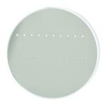
The photograph above is a protected aluminum-coated mirror after LIDT testing. In this particular test, it handled  $0.43\ Jcm^2\ (1064\ nm, 10\ ns\ pulse, 10\ Hz, \emptyset 1.000\ mm)$  before damage.
