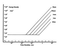
LIDT in energy density vs. pulse length and spot size. For short pulses,
