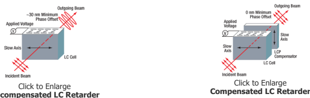
Click to Enlarge Uncompensated LC Retarder Click to Enlarge Compensated LC Retarder Figure 2: The minimum retardation of uncompensated liquid crystal retarders is \sim 30 nm. Our compensated LC retarders include a liquid crystal polymer compensator with a fixed retardation and slow axis that is orthogonal to that of the variable LC cell. This enables our compensated retarders to achieve a minimum retardance of 0 nm.
