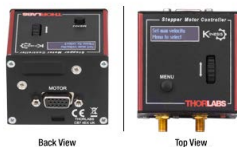
Click to Enlarge Back and Top Views of the KST101 K-Cube (See the Pin Diagrams Tab for More Information)
