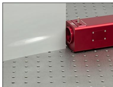
The photo above shows light from an SLS201L 2796 K tungsten-halogen source with an FGT200 Ø25.0 mm filter installed. For a plot of the power output with and without a filter, please see the *Conversion Values* tab.
